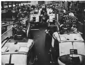
HU-1A Iroquois assembly line at Bell Helicopter Corp.'s Renton, Wash. plant indicates high production rate for the Lycoming T-55 powered Army helicopter. Detail component assemblies are made up on line at left, then fed into two major assembly pits at left, rear.
